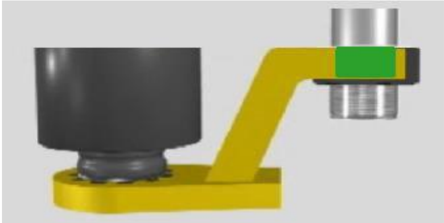
Figure 1.5 Correct reaction point 正确的反力点
